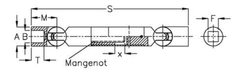
A = 100 F = 54 Longitudinal ribs = 20x54x62M = 145.0 MD max N m = 1250 s = 900 T = 80
